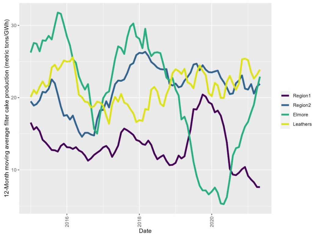
Figure 9.4. Twelve-month moving average of filter cake solid waste tonnage per GWh produced and disposed of at the Desert Valley Monofill from the BHER SS-GF geothermal power plants.
