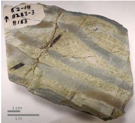
Figure A4.9. Epidotized mudstone from 2485 m (8153 ft) depth in the State 2-14 drill core.
